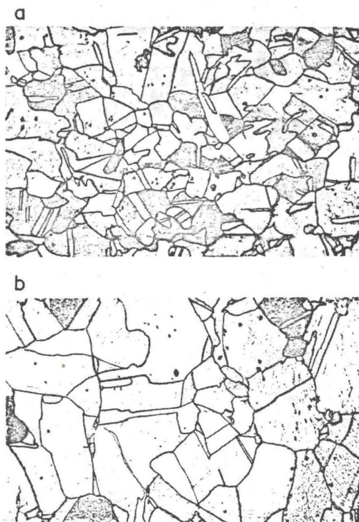
FIG. 5. Microstructures of copper after shock loading at 500° (a) and 400° (b). Cooling in water; \times 100 .
